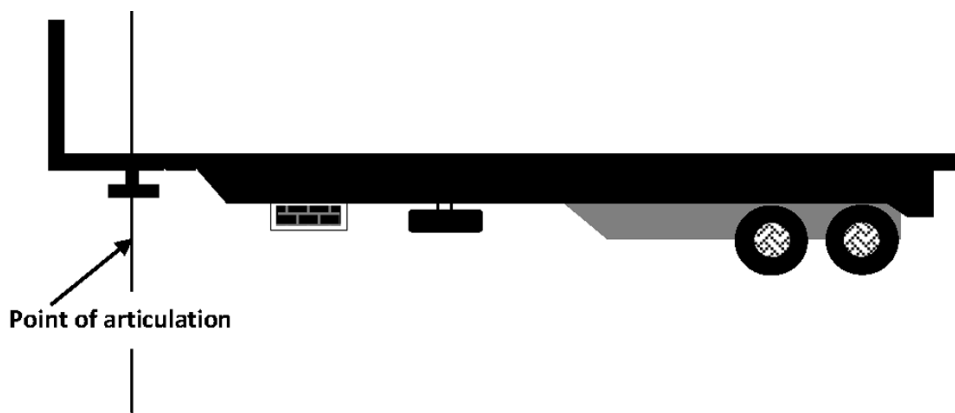
Point of articulation—fifth wheel on a prime mover
