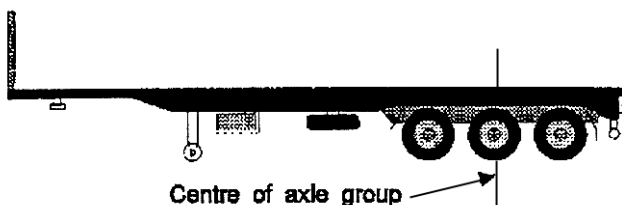
Centre of a typical tri-axle group
