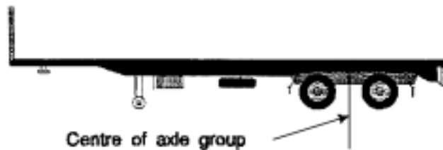
Centre of a typical tandem axle group fitted with an equal number of tyres on each axle
