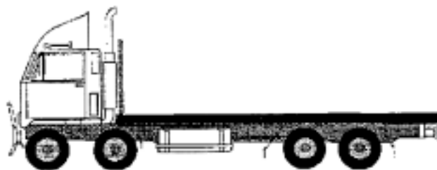
Typical twinsteer axle group on a motor vehicle
