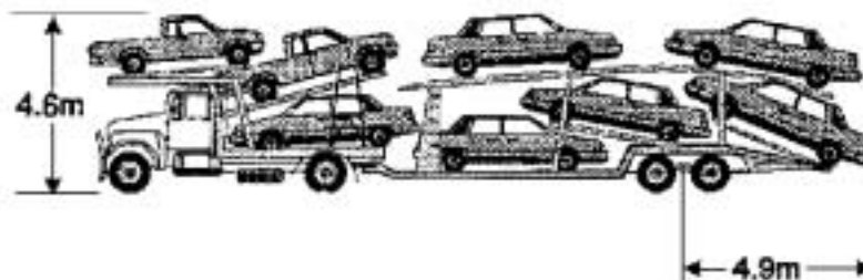
Height limit and rear overhang limit of a loaded car carrier
