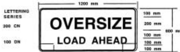
Illustration of a warning sign for a pilot vehicle
