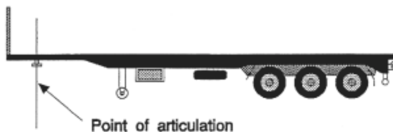
Point of articulation—kingpin for fifth wheel
