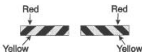
An alternative pattern for rear marking plates
