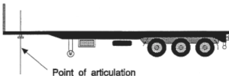
Point of articulation—kingpin for fifth wheel
