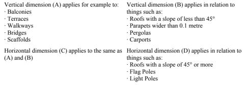
TABLE 2: Clearance distance for aerial lines (excluding service lines, other cable systems and aerial lines within substations)
