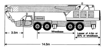
Rigid mobile crane showing dimension limits
