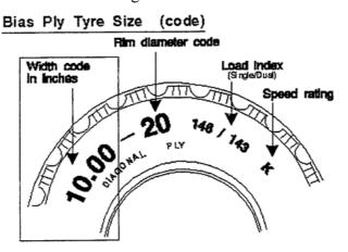
Position of width code marking on diagonal or bias type tyre
