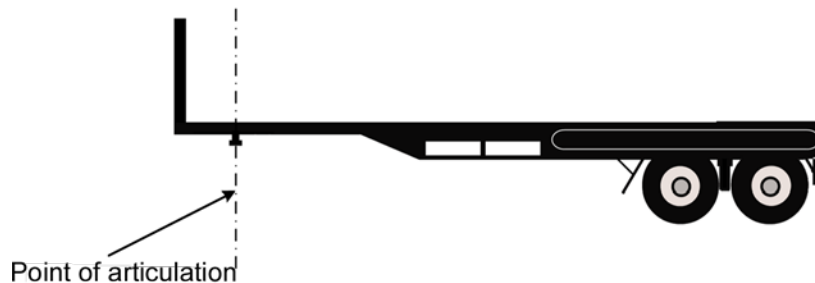
Point of articulation - kingpin for fifth wheel
