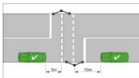
Measurement of distance—bicycle crossing lights
