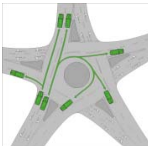
Roundabout with 5 entry points
