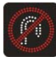
No U-turn sign (Variable illuminated message sign)
