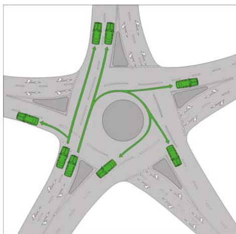
Roundabout with 5 entry points
