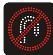
No U-turn sign (Variable illuminated message sign)
