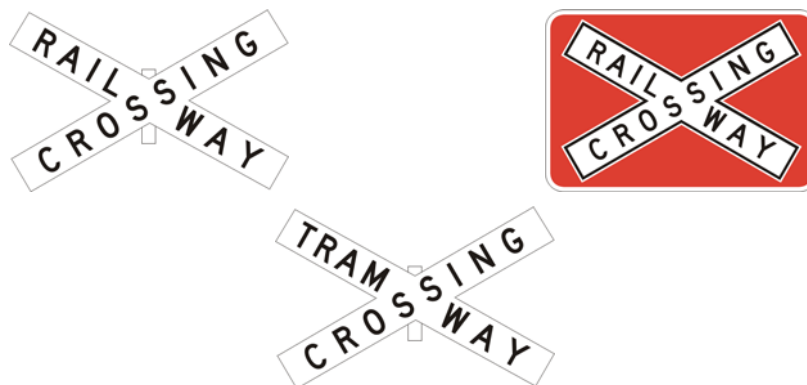
Level crossing signs
