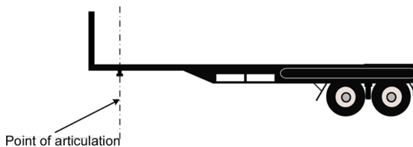
Point of articulation - kingpin for fifth wheel
