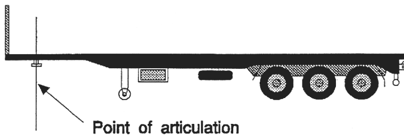
Point of articulation—kingpin for fifth wheel
